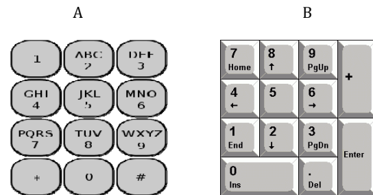
Fig 1. Example of two keypad layouts, panel A is the TEL layout, and panel B is the ADD layout.
